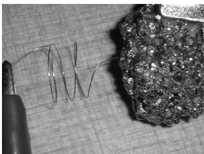
Figure 1: Iron Pyrites with #30 copper wire catwhisker.
